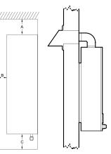
4"single wall venting only. Use stainless steel (AL29-4C) or galvanized pipe of 26 minimum gauge must be used. Each connection must be properly sealed.
